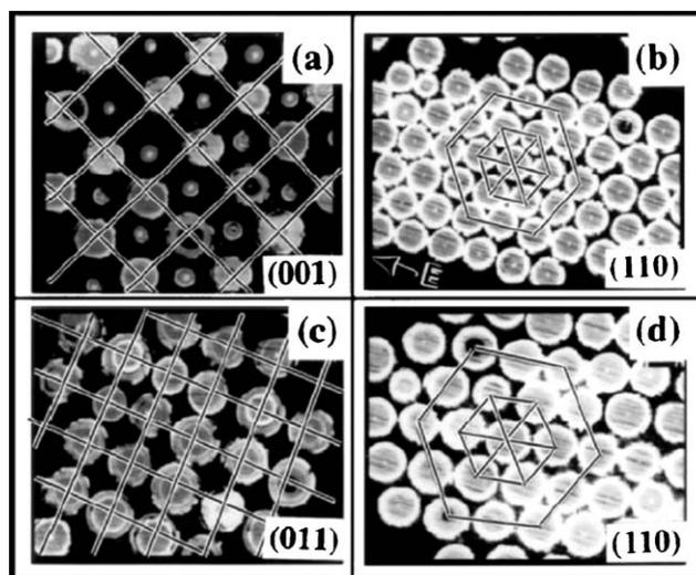
**Fig. 3** (a) and (b) BCT structure formed by multiply-coated microspheres under an electric field ( $2 \text{ kV mm}^{-1}$ ). The structure is frozen in epoxy and visualized through cross-sectional SEM micrographs. (c) and (d) are the signatures of a FCC structure formed by the same multiply-coated microspheres under a crossed electric field ( $2 \text{ kV mm}^{-1}$ ) and magnetic field (54 G).
