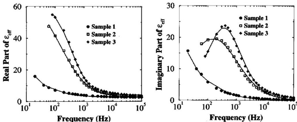
Fig. 5 The real and imaginary parts of the effective dielectric constants for the three samples plotted as a function of frequency. The symbols represent the experimental measurements and the lines are fitted theoretical calculations. The free material parameters are determined by the fittings.
