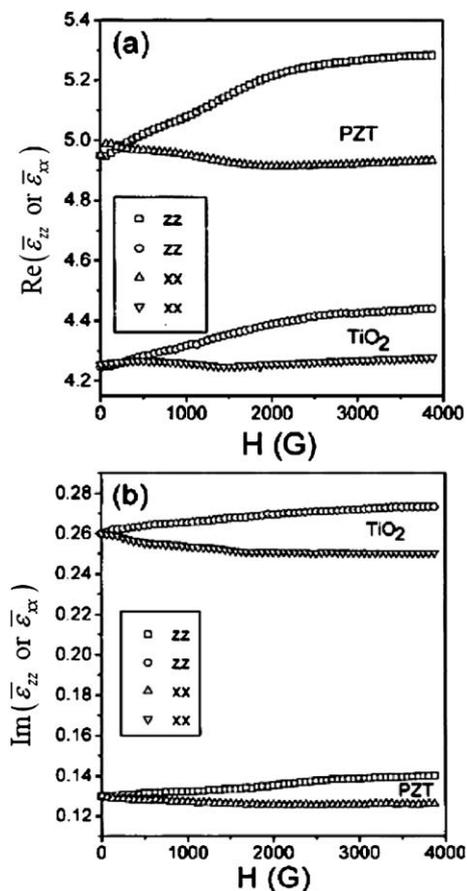
**Fig. 10** Dependences of real (a) and imaginary (b) parts of the dielectric constant on applied magnetic field strength. Here the volume fraction is 0.27, and the frequency of the LCR meter is fixed at 1 kHz.
