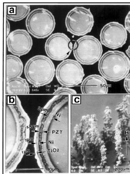
**Fig. 2** (a) Cross-sectional SEM picture of the coated spheres. The apparent size variation is caused by deviation of the spheres' centers from the cutting plane. The arrow points to a circular region detailed in (b), which shows in detail the thickness of the four coatings. From the inside out:  $2 \mu\text{m}$  Ni,  $1.5 \mu\text{m}$  PZT,  $1 \mu\text{m}$  Ni, and finally  $1 \mu\text{m}$   $\text{TiO}_2$ . (c) The coated EMR spheres under the influence of a small magnetic stirrer.
