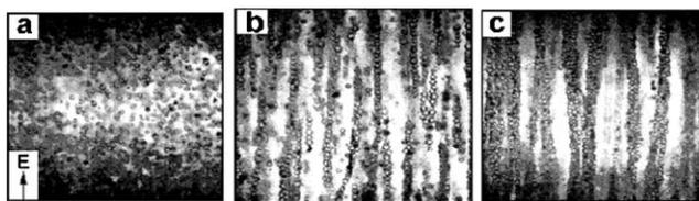
**Fig. 1** The structural evolution of dielectric microspheres under an increasing electric field, from (a) no field, to (b) a moderate field of  $500 \text{ V mm}^{-1}$ , to (c) a strong field of  $900 \text{ V mm}^{-1}$ . Here the ER fluid consists of 1.5 micron glass spheres suspended in silicone oil.
