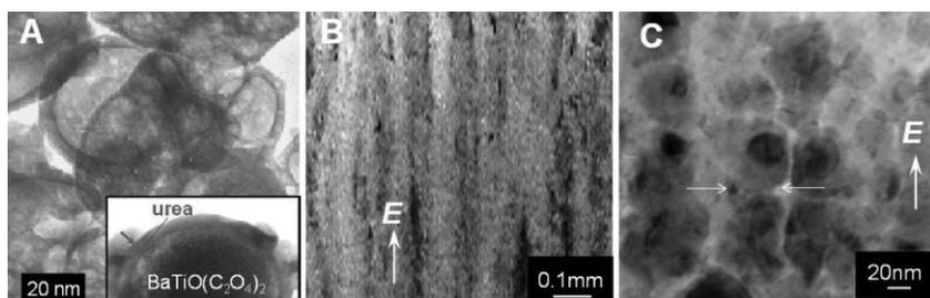
**Fig. 11** Images of nanoparticles in GER suspensions. (a) TEM image of coated nanoparticles. Urea coatings are clearly seen. (b) Optical microscope image of a sample prepared in epoxy, solidified under an applied field  $E$  of  $2 \text{ kV mm}^{-1}$ . Columns aligned along the field direction are visible. (c) TEM image of a section of the column shown in (b). The arrows indicate one of the flattened interfaces.
