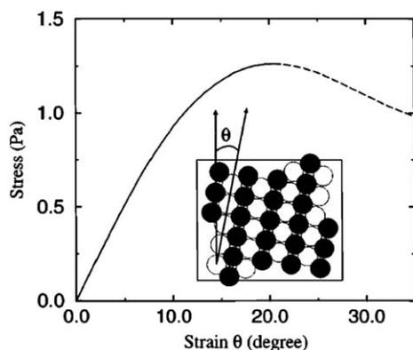
**Fig. 4** Calculated stress, in units of Pascals, plotted as a function of strain, *i.e.*, the tilt angle  $\theta$  as defined in the inset. The dashed line indicates the unstable regime. The maximum stress is defined as the static yield stress. Here the curve is calculated with  $\epsilon_1 = 2.7$ ,  $\epsilon_s = 8.4 + 0.43i$ , the volume fraction of spheres is 22%, and the applied field is  $1.3 \text{ kV mm}^{-1}$ .
