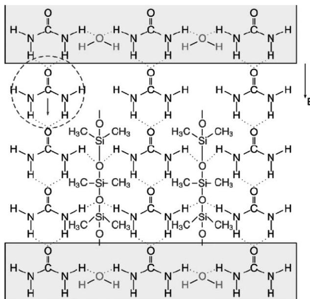
**Fig. 14** A schematic hydrogen bonding (indicated by the dotted lines) network favoring the formation of parallel alignment of urea molecular dipoles. The urea molecular dipole unit is indicated by the dashed line, with direction as shown.
