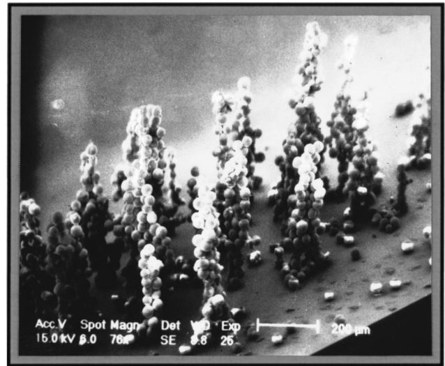
FIG. 3. SEM micrograph of columns of MBPZT microspheres suspended by a small magnetic field.
