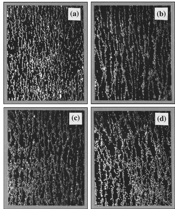
FIG. 5. The patterns formed by glass microspheres with different water contents. The water contents in (a), (b), (c), and (d) are 0, 0.254, 1.673, and 5.348 wt. %, respectively. The applied field strength is 700 V/mm.
