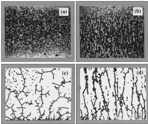
FIG. 4. Development of the pattern transition performed with PMMA-based microspheres, where (a) is pure PMMA, (b) is PMMA with a thin layer of nickel coating, (c) is PMMA coated with a good conducting nickel layer, and (d) is PMMA double coated with an inner conducting and outer insulating layer. The field strength is fixed at 600 V/mm.
