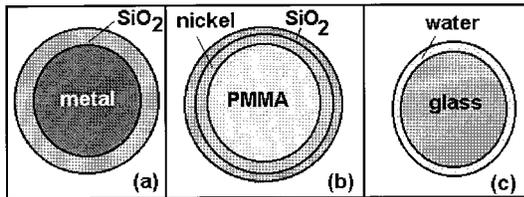
FIG. 1. Microspheres with different coating materials.
