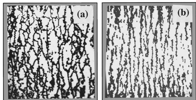
FIG. 3. Pattern transition when an insulating layer is coated on the copper microsphere, where (a) is a pure copper microsphere and (b) is the microsphere after coating.
