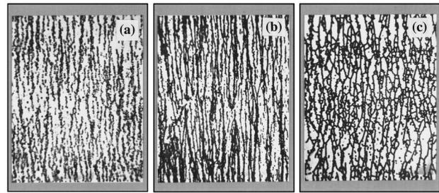
FIG. 2. Pattern formations performed with different kinds of microspheres, where (a), (b), and (c) show the patterns formed by  $\text{SrTiO}_3$ , Si, and Cu microspheres, respectively.
