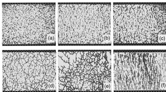
FIG. 2. Development of the two-dimensional structure of a metal/oil ER fluid containing 0.2 volume fraction of indium spheres with increasing electric field. (a)  $E=0$ , (b)  $E=200\ \text{V/mm}$ , (c)  $E=500\ \text{V/mm}$ , (d)  $E=700\ \text{V/mm}$ , (e) and (f) are the structural patterns formed with metal and glass spheres when the electric field is applied suddenly. In both of these cases, the experiments are performed under the same conditions.
