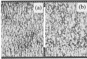
FIG. 4. The structural changes when the electric field strength is below and above a certain threshold value.
