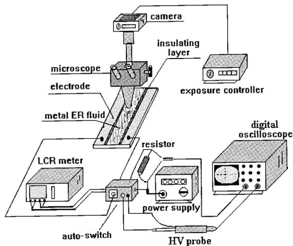
FIG. 1. Schematic diagram showing the experimental setup.
