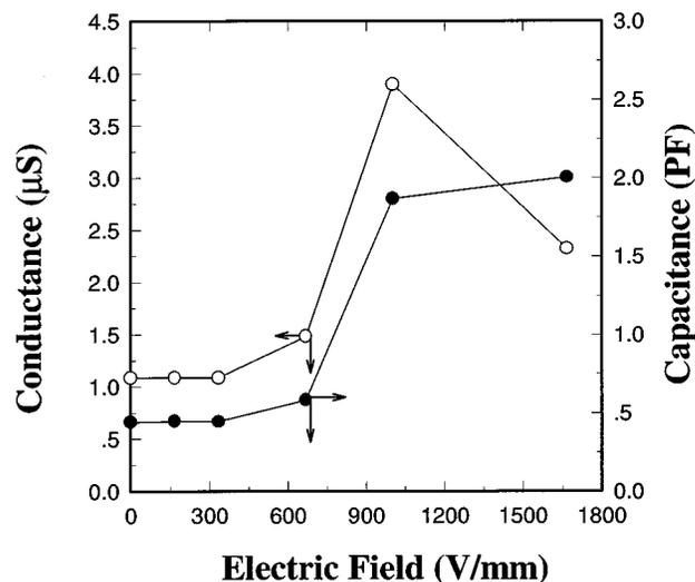
FIG. 3. Dielectric properties and energy of the metal ER fluid as the electric field was increased. The measured frequency was fixed at  $200\ \text{kHz}$ . The volume of the ER fluid cell used here is  $70\ \text{mm} \times 2\ \text{mm} \times 1\ \text{mm}$ .
