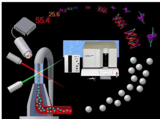
**Fig. 13** Luminex xMAP system and components illustration adapted from [228]. The four main components of the xMAP system are shown, clockwise from top-right: biomolecular reactants; fluorescently color-coded microspheres; fluidics and optics; and high-speed digital signal processing. The Luminex 100 analyzer with XY platform and sheath delivery system is pictured in the center
