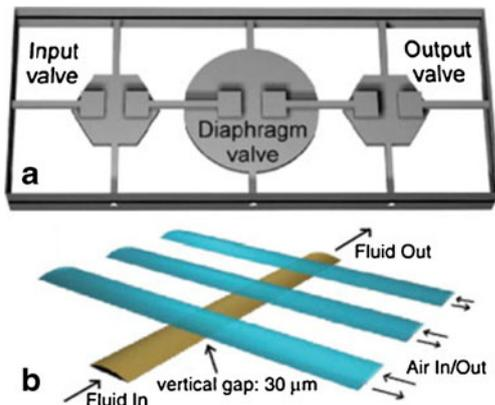
**Fig. 7** **a** an oblique view of the three-layer pneumatic diaphragm micropump. Adapted from [201]. **b** A 3D scale diagram of a pneumatic peristaltic micropump. Adapted from [181]
