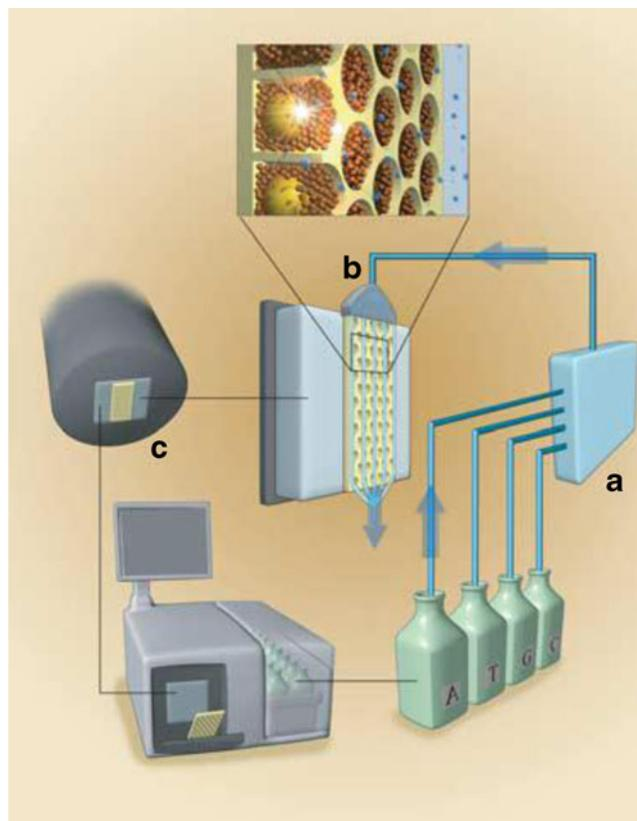
**Fig. 14** Four hundred fifty-four technology sequencing instrument illustration adapted from [234]. The sequencing instrument consists of the following major subsystems: a fluidic assembly (a), a flow chamber that includes the well-containing fibre-optic slide (b), a CCD camera-based imaging assembly (c), and a computer that provides the necessary user interface and instrument control
