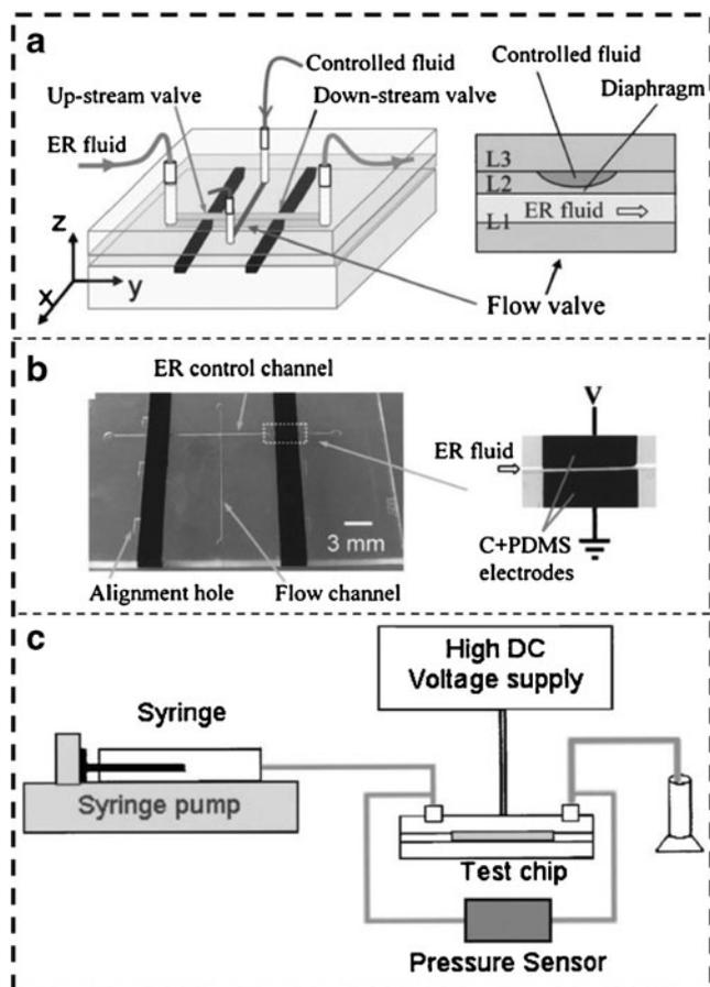
**Fig. 5** Design and fabrication of micro-ER valve. Adapted from [184]. **a** Design of four-port valve chip. Right: cross-section of the different layers forming the flow valve; L1 is the ER fluid channel layer, L2 the controlled flow channel layer, and L3 the cover layer. **b** Optical photograph of fabricated ER valve chip. Right: top-view image of the planner electrodes and the ER fluid channel. **c** Experimental setup for microvalve testing
