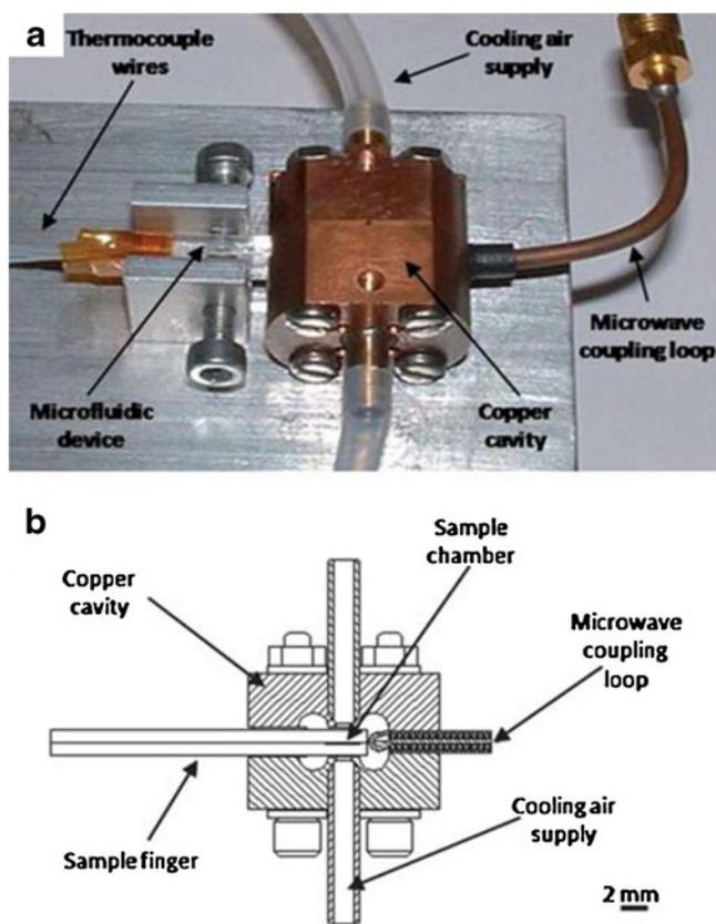
**Fig. 3** Photograph (a) and schematic cross-section (b) of the re-entrant cylindrical microwave cavity from Shaw et al. [46]
