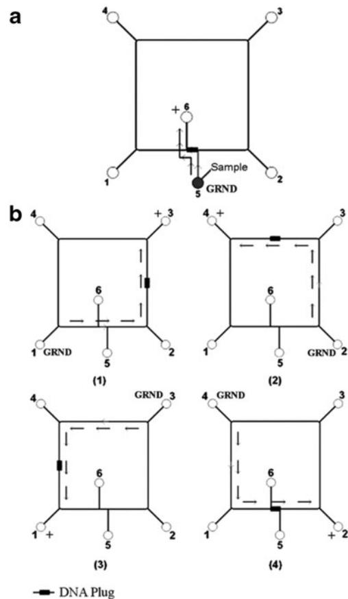
**Fig. 9** Diagrammatic principle of electrokinetic synchronized cyclic continuous flow PCR process. **a** Sample injection; **b** Sample cycling. Adapted from [205]
