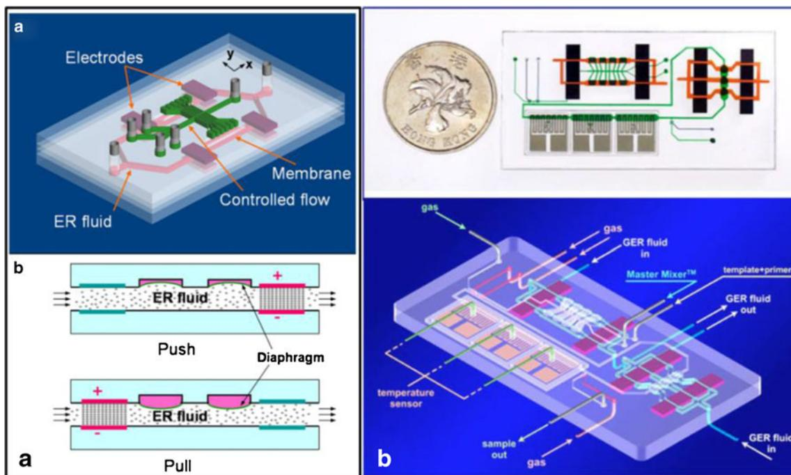
**Fig. 11** **a** Scheme of mixer construction. Adapted from [219]. **(a)** Schematic picture showing the PDMS active mixer design and construction. The overall chip size is 3 cm by 1.5 cm. **(b)** Schematic illustration showing the working principle for the push and pull ER valve, for one
