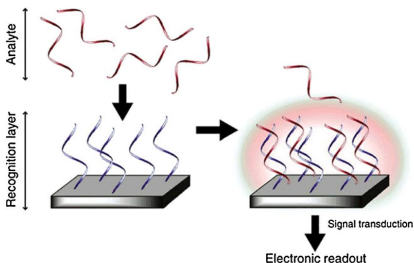
**Fig. 12** Target DNA is captured at the recognition layer and the resulting hybridization signal is transduced into a usable electronic signal for display and analysis. In the case of electronic and electrochemical biosensors, signal transduction is greatly simplified, because the incoming signal is already electronic in origin [223]
