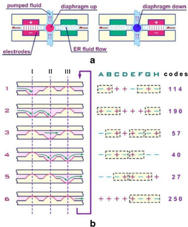
**Fig. 8** **a** The principle of ER valve's operation is illustrated schematically by showing the deformation of a single diaphragm via pumped ER fluid. The diaphragms' pumping sequences and their corresponding signals are shown in (b). Adapted from [204]
