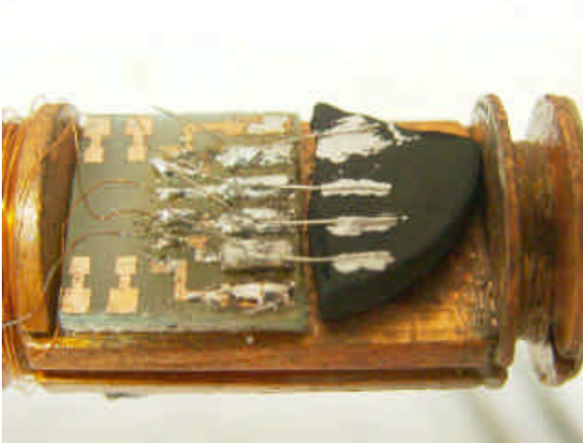
The 4 point probe set-up with a piece of YBCO, to be immersed in liquid nitrogen for testing
