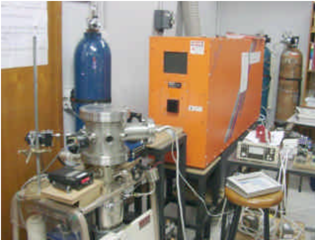
KrF Excimer Laser used in PLD
